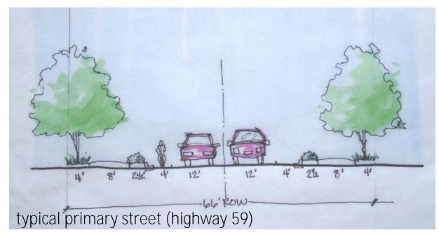
primary vehicular pedestrian route has 66**'** right-of-way. existing Within this right-of-way, the vehicular lanes have maintained their existing width and a new designated bike lane with curb and gutter has been added. A landscaped verge has been added to serve as buffer between the new 8' sidewalk.
